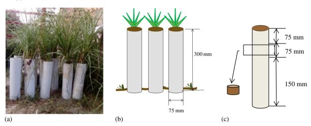
Figure 1. Vetiver plantation scheme (a) Vetiver grass planted in PVC pipe; (b) Schematic diagram of vetiver plantation in PVC pipe; (c) Schematic diagram of retrieving undisturbed sample from PVC pipe
