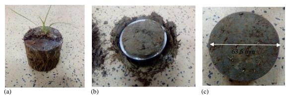
Figure 2. Steps of sample preparation (a) Soil retrieved from pipe, (b) Collection of 62.5 mm dia specimen from 75 dia soil sample, (c) Specimen in probing ring
